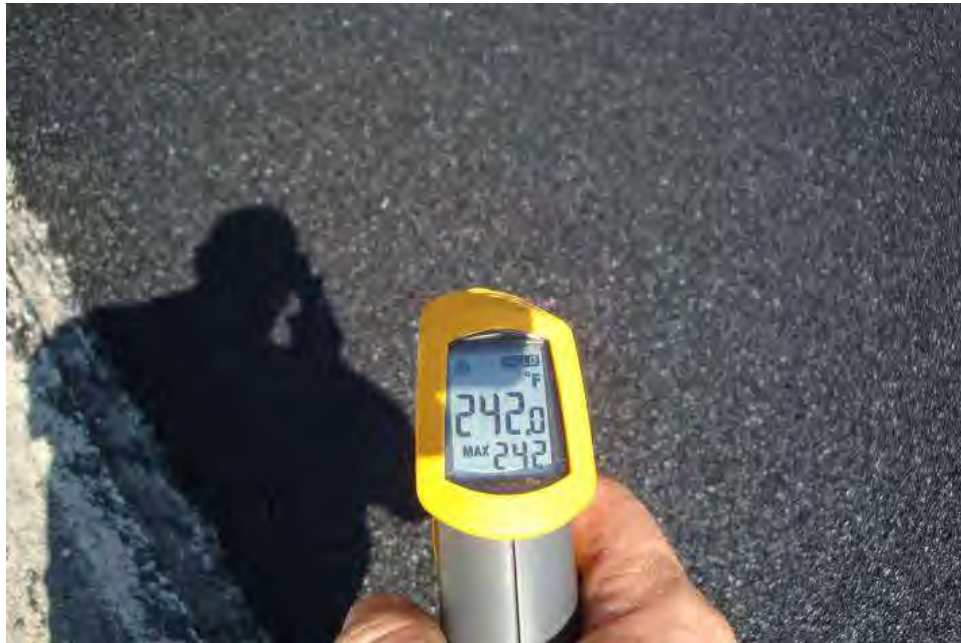
FIGURE 4 Route 50 Gasconade County 12.5-mm NMA S WMA RAP and RAS – Low Temperatures
