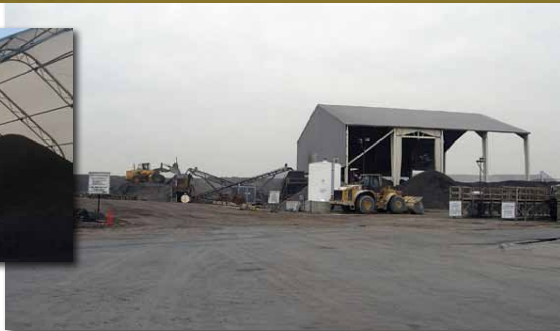
Covering stockpiles helps keep moisture to a minimum, which reduces drying times and temps, thus reducing the risk of blue smoke generation. Photos courtesy of Murphy Pavement Technology, Chicago.
